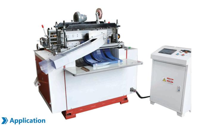
Die cutting plastic STRAIGHT shirt collar bands ONLY, collar supports,collar strips in PP, PVC, PET, PS material.
